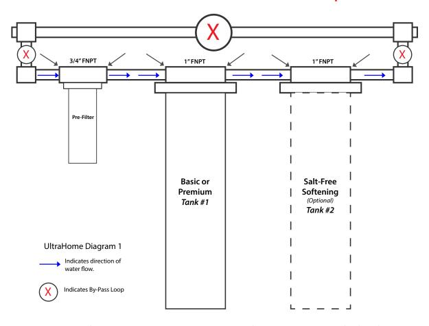
All AlkaViva non-backwashing filtration systems come with sediment pre-filtration to extend the life of the filter(s). The sediment pre-filter will always be the first stage that water flows through.
